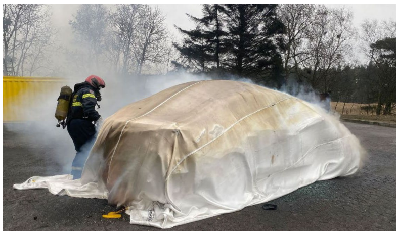
Figure 9. EV fire blanket deployed on a vehicle (from Hessels and Geertsema, 2023).
