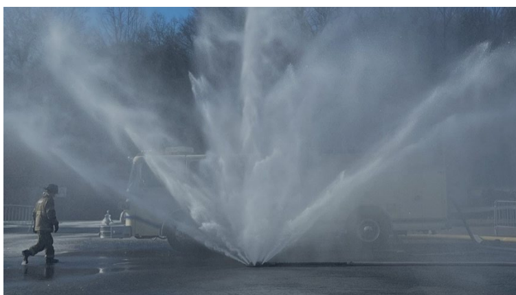
Figure 10. Spray pattern from an undercar cooling nozzle (from Turtle™ Fire Systems, 2023).
