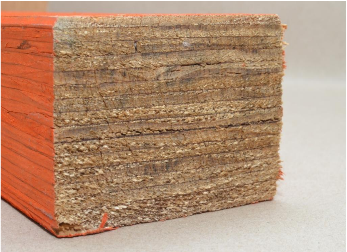
Photo showing timber formwork beam.
