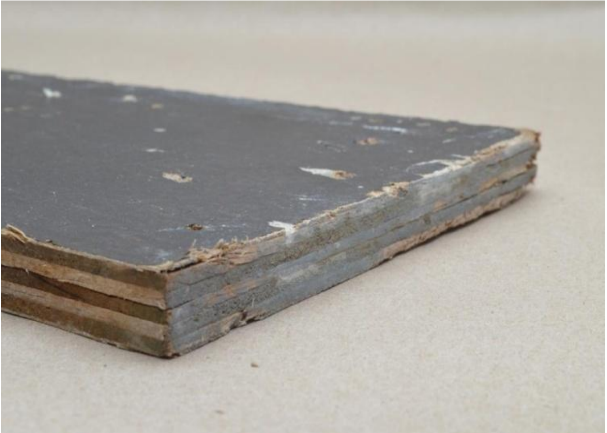
Photo showing timber plywood formwork sheet.
