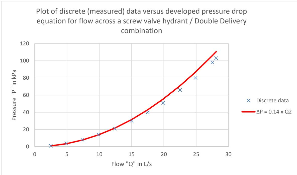
Figure 11: Plot of discrete (measured) data versus developed pressure drop equation for flow across a screw valve hydrant / double delivery combination
