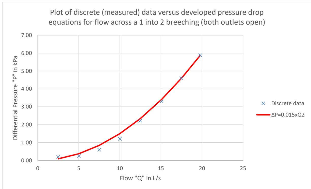
**Figure 5: Plot of discrete (measured) data versus developed pressure drop equations for flow across a 1-into-2 breaching (both outlets open)**
