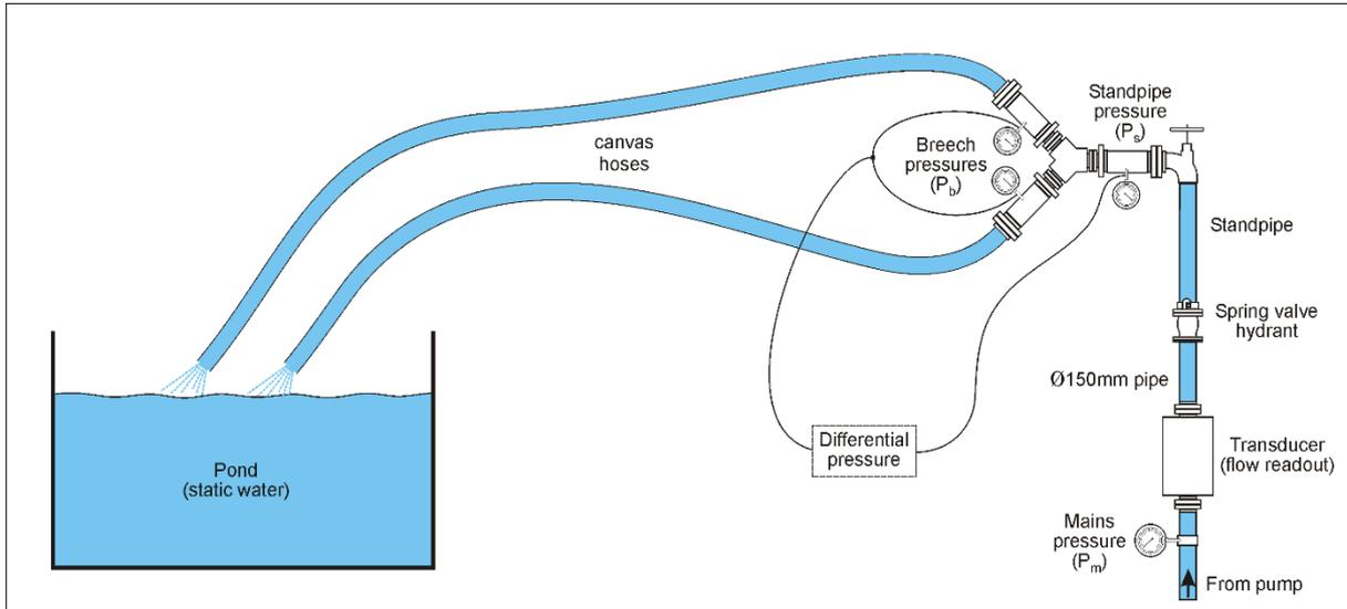
Figure 4: MHL Figure 2-10 – Test C2 set-up for flow across a 1-into-2 breaching
