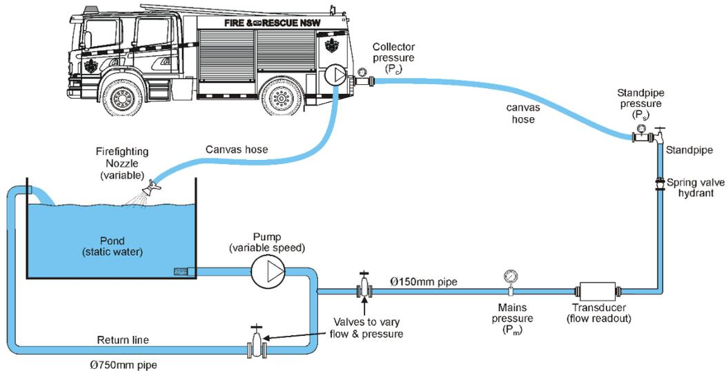
**Figure 1: MHL Figure 2-7 : Tests A5 and A6 configuration**
