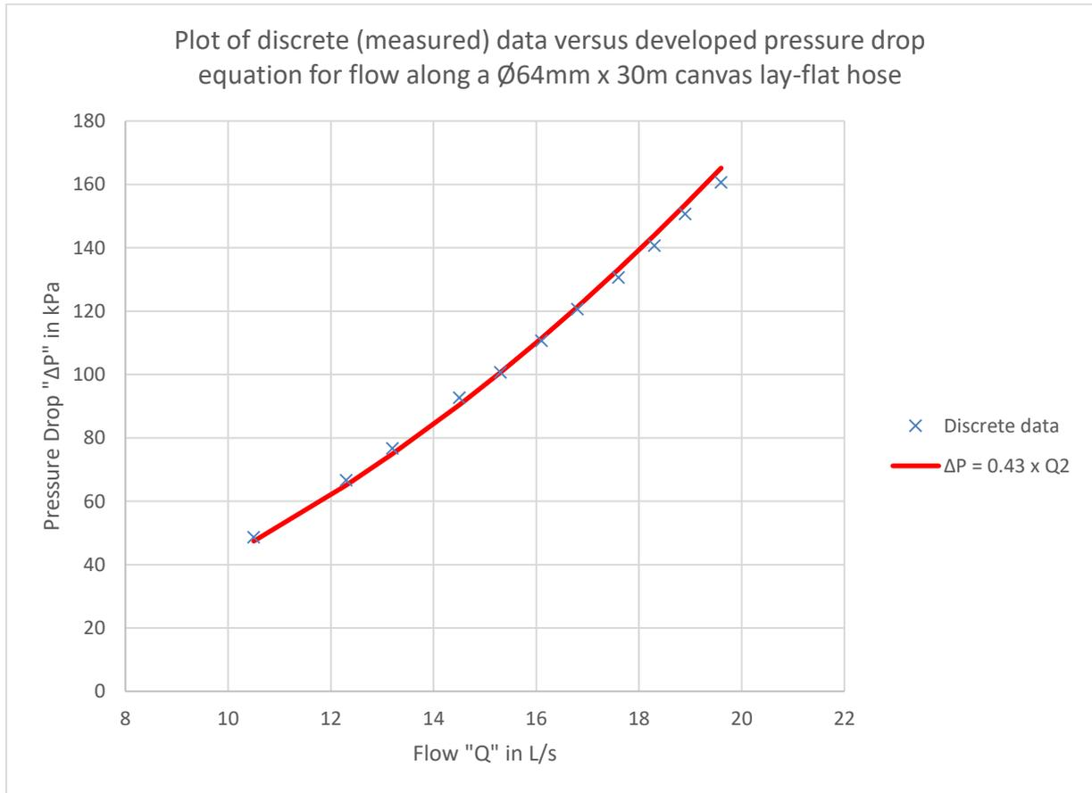
**Figure 10: Plot of discrete (measured) data versus developed pressure drop equation for flow along a Ø64mm x 30m canvas lay-flat hose**
