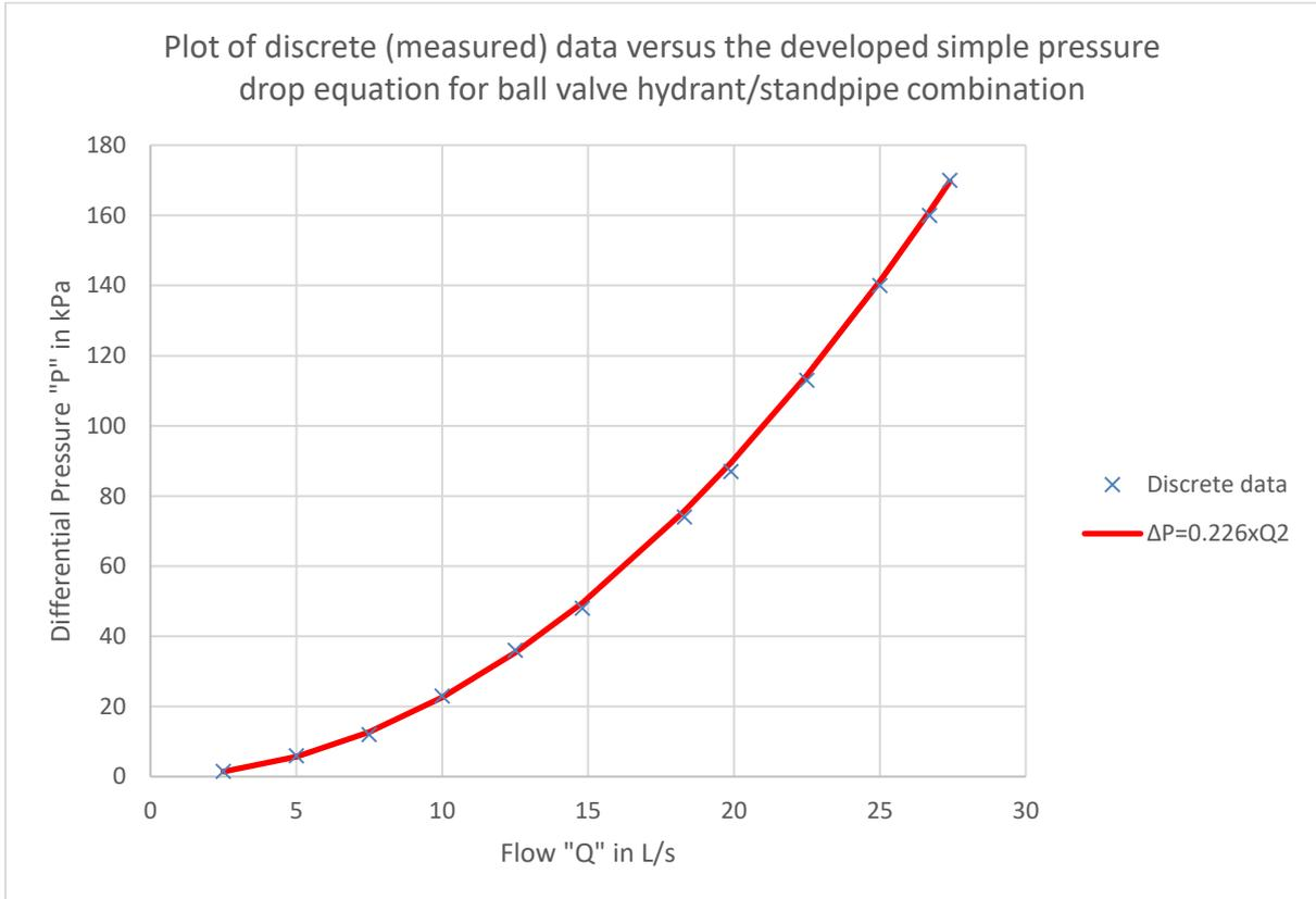
**Figure 3** Plot of discrete (measured) data versus the developed simple pressure drop equation for ball valve hydrant/standpipe combination
