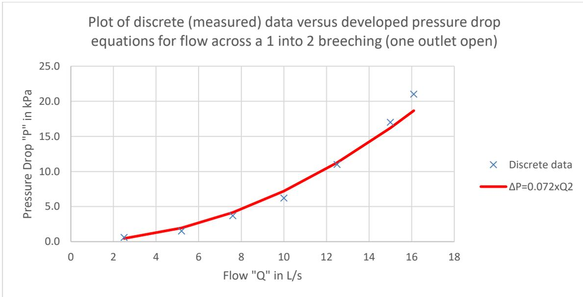
**Figure 6: Plot of discrete (measured) data versus developed pressure drop equations for flow across a 1-into-2 breaching (one outlet open)**
