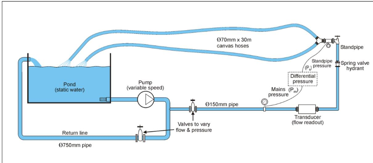
Figure 2: MHL Figure 2-9: Test C1 (and Test C5) set-up, spring valve hydrant / standpipe
