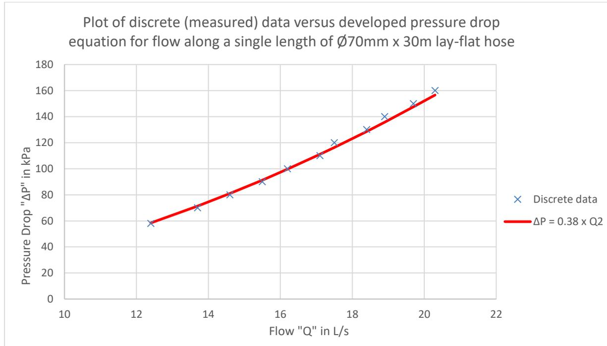
Figure 8: Plot of discrete (measured) data versus developed pressure drop equation for flow along a single length of Ø70mm x 30m lay-flat hose
