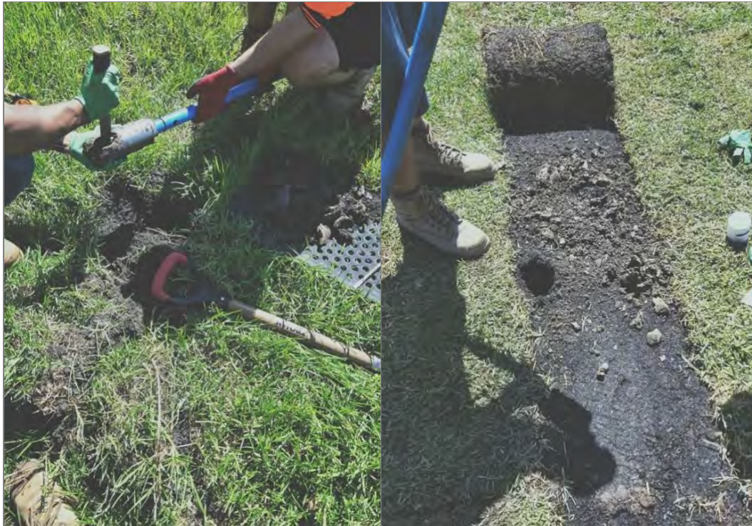
Photo 9: Soil sampling from freshly turfed area (S16a – 19 Feb 2020)
